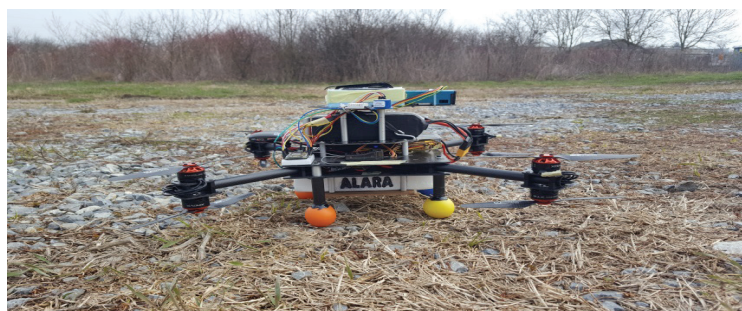
Unmanned aircraft (UAV; colloquially drone) and the measuring system ALARA UAV-IPPSO
