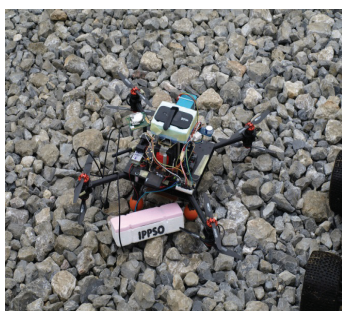
Unmanned aircraft (UAV; colloquially drone) and the measuring system ALARA UAV-IPPSO
